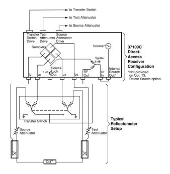
A Reflectometer test set is available as a special option for the 37100C. It contains the transfer switch, both attenuators and couplers. It also offers two bias tees and a front panel amplifier loop for active device testing. As compared to a 37300C VNA, the output power and hence the dynamic range are degraded by 10 dB typically.
